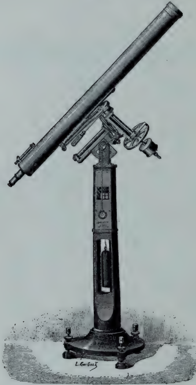
EQUATORIAL CONSTRUCTED TO ALLOW OF CONSIDERABLE VARIATION IN LATITUDE.
